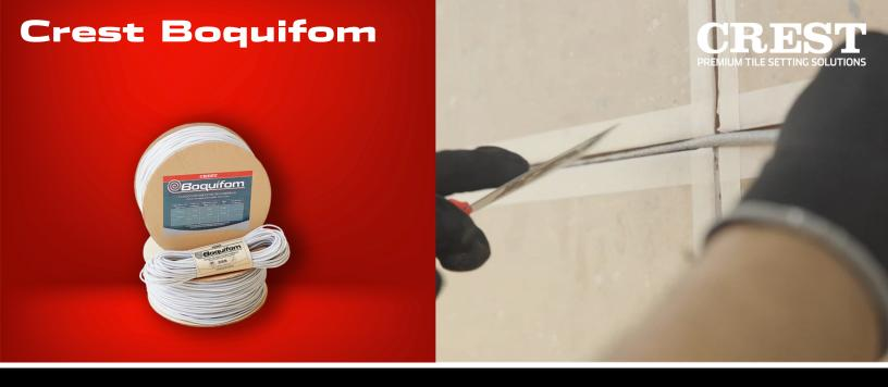
CREST Boquifom® is a backing material that is inserted into the joint, it is a low-density, closed-cell polyethylene foam cord, specially designed to be placed in expansion or contraction joints, before they are sealed.
